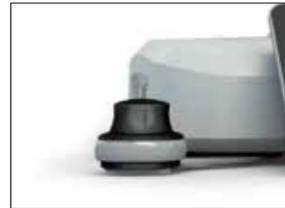
Digital joystick is optional for manual alignment and focusing.
